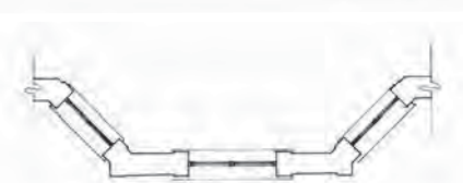
Chamfered bay window in elevation and plan with appropriate proportions and details.
