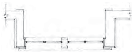
Square bay window in elevation and plan with appropriate proportions and details.
