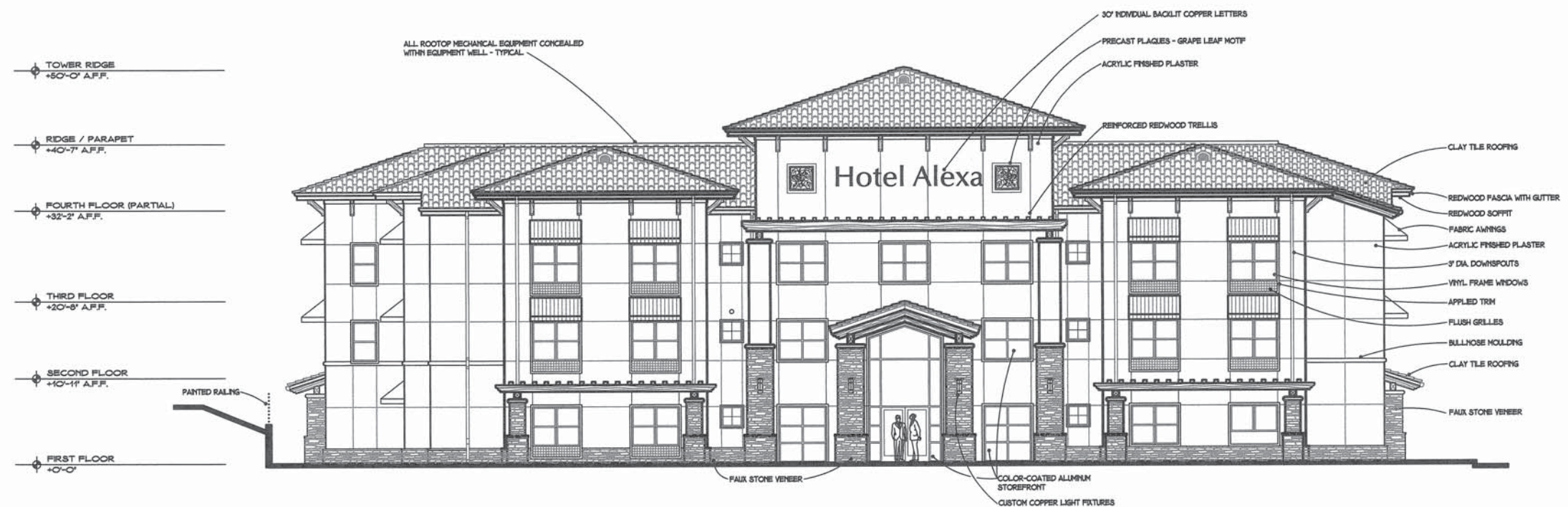
South Elevation (Front - View From Alexa Court)
