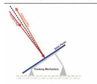
Incident and reflected rays of light that would result from a optimally oriented solar panel on a variable tilt single axis tracking mechanism.
