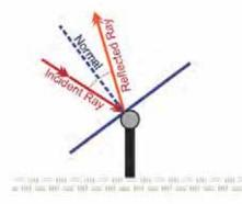
Incident and reflected rays of light that would result from the fixed tilt single axis tracker array.
