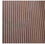
EXTERIOR TOWER WALLS: 1 1/2" DEEP VERTICAL PRE-FINISHED METAL SIDING RUST COLOR TO MATCH EXISTING
