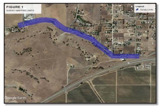
The aerial topographic mapping together with the supplemental mapping, Right of Way and easement delineation included in this task will be compiled to form the survey base map used as the basis of preliminary design and engineering. Additional survey field work to densify specific areas of conform or other needs may be incorporated in a final design phase if the project moves forward beyond this preliminary phase.
