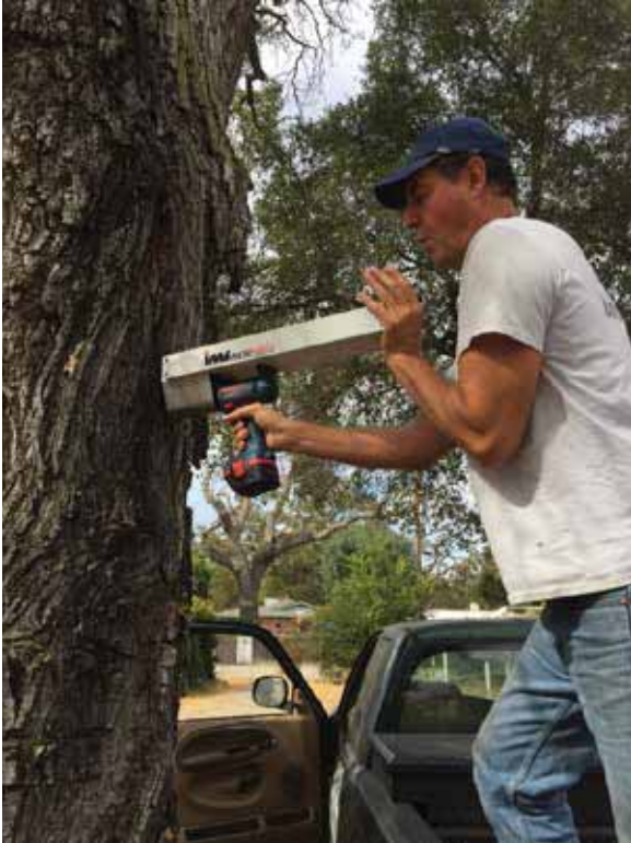
October 13, 2016 resistograph test of tree by arborist Chip Tamagni
