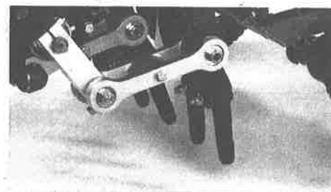
Reciprocating tines provide vertical coring action, punching straight in and out without tearing the turf, offering quality on par with golf courses.
