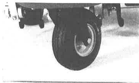
4. Liquid front caster wheel allows the machine to maneuver with near zero-turn capability.
